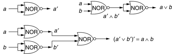
Figure 2.30. Basic operations constructed from NOR gates.
