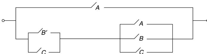
Figure 2.24. Series-parallel circuit.
