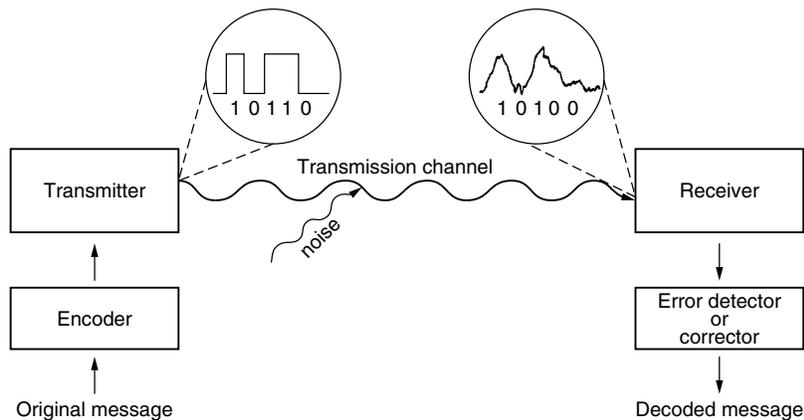
Figure 14.2. Block diagram for error detection or correction.
