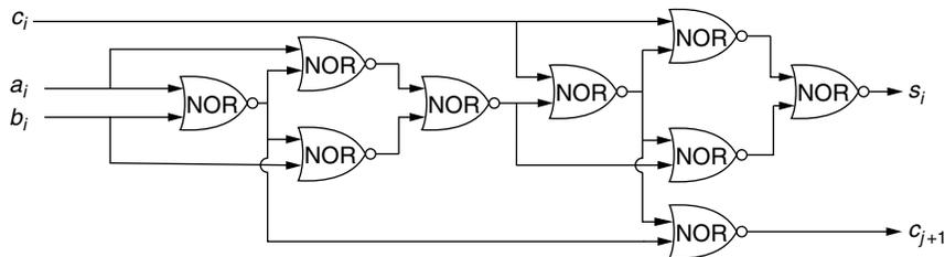
Figure 2.31. Full adder using NOR gates.
