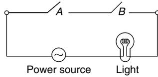
Figure 2.10. Series circuit.
