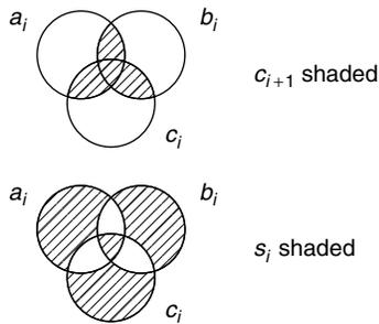
**Figure 2.27.** Venn diagrams for a full adder.
