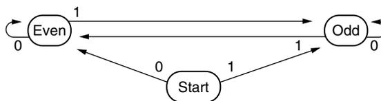
Figure 7.4. State diagram of the parity checker.
