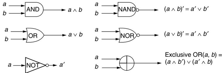
Figure 2.29. Transistor gates.
