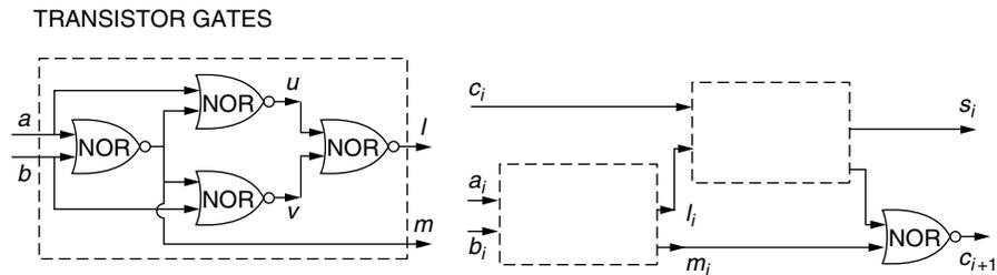
Figure 2.32. Component parts of the full adder.
