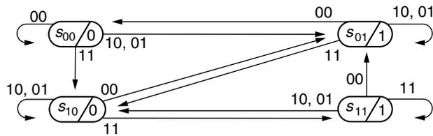
Figure 7.12. State diagram of the serial adder.
