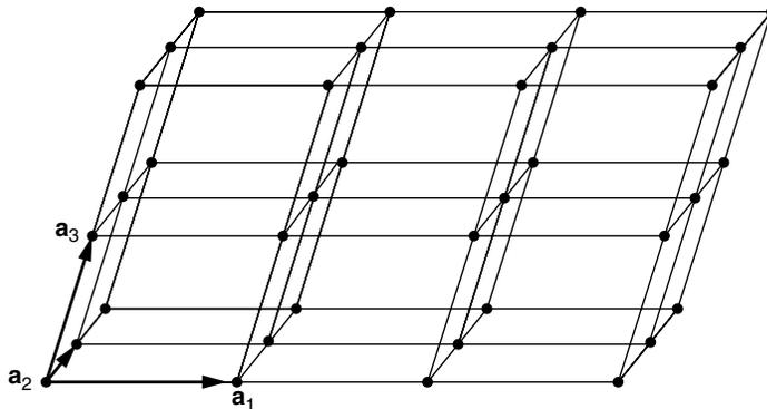
Figure 5.10. Crystalline lattice.
