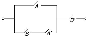
Figure 2.12. Series-parallel circuit.
