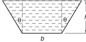
The figure shows the cross section of a channel carrying water. Determine  $h$ ,  $b$  and  $\theta$  that minimize the length of the wetted perimeter while maintaining a cross-sectional area of  $8 \text{ m}^2$ . (Minimizing the wetted perimeter results in least resistance to the flow.) Use the Fletcher-Reeves method.
