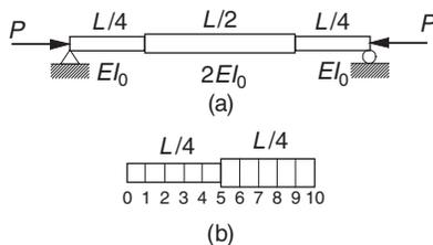
The simply supported column in Fig. (a) consists of three segments with the bending rigidities shown. If only the first buckling mode is of interest, it is sufficient to model half of the beam as shown in Fig. (b). The differential equation for the lateral displacement  $u(x)$  is
