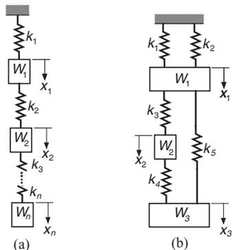
13. ■ The displacement formulation for the mass–spring system shown in Fig. (b) results in the following equilibrium equations of the masses:
