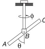
The bar  $ABC$  is attached to the vertical rod with a horizontal pin. The assembly is free to rotate about the axis of the rod. In the absence of friction, the equations of motion of the system are
