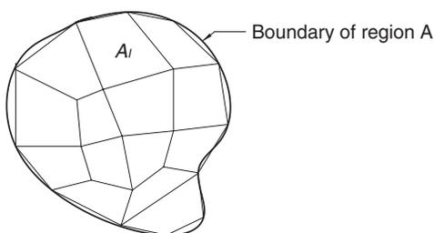
Figure 6.6. Finite element model of an irregular region.
