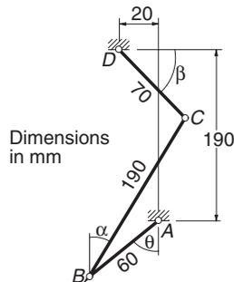
Geometric analysis of the linkage shown resulted in the following table relating the angles  $\theta$  and  $\beta$ :
