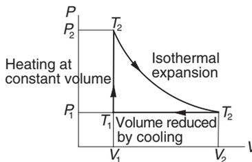
The figure shows the thermodynamic cycle of an engine. The efficiency of this engine for monatomic gas is
