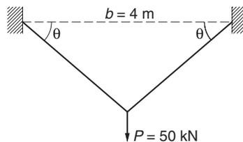
Each member of the truss has a cross-sectional area  $A$ . Find  $A$  and the angle  $\theta$  that minimize the volume
