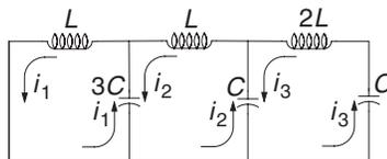
(1) Show that the analysis of the electric circuit shown leads to a matrix eigenvalue problem. (2) Determine the circular frequencies and the relative amplitudes of the currents.
