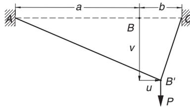
The elastic cord  $ABC$  has an extensional stiffness  $k$ . When the vertical force  $P$  is applied at  $B$ , the cord deforms to the shape  $AB'C$ . The potential energy of the system in the deformed position is
