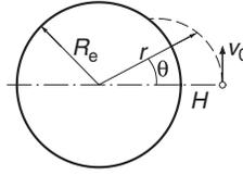
A spacecraft is launched at an altitude  $H = 772$  km above sea level with the speed  $v_0 = 6700$  m/s in the direction shown. The differential equations describing the motion of the spacecraft are
