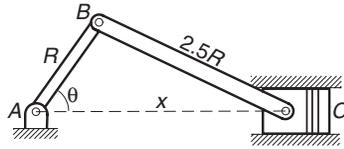
The crank  $AB$  of length  $R = 90$  mm is rotating at the constant angular speed of  $d\theta/dt = 5000$  rev/min. The position of the piston  $C$  can be shown to vary with the angle  $\theta$  as
