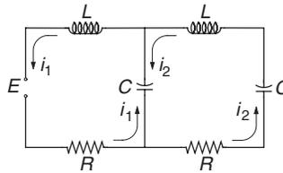
The constant voltage source  $E$  of the circuit shown is turned on at  $t = 0$ , causing transient currents  $i_1$  and  $i_2$  in the two loops that last about 0.05 s. Plot these currents from  $t = 0$  to 0.05 s, using the following data:  $E = 9$  V,  $R = 0.25 \Omega$ ,  $L = 1.2 \times 10^{-3}$  H and  $C = 5 \times 10^{-3}$  F. Kirchoff's equations for the two loops are
