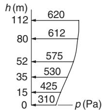
The pressure of wind was measured at various heights on a vertical wall, as shown on the diagram. Find the height of the pressure center, which is defined as
