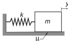
Consider the mass–spring system where dry friction is present between the block and the horizontal surface. The frictional force has a constant magnitude  $\mu mg$  ( $\mu$  is the coefficient of friction) and always opposes the motion. The differential equation for the motion of the block can be expressed as
