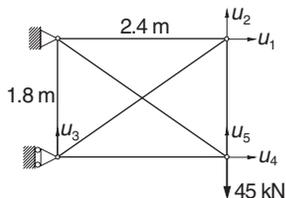
The displacement formulation for a plane truss is similar to that of a mass–spring system. The differences are: (1) the stiffnesses of the members are
