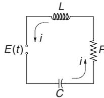
The differential equations governing the loop current  $i$  and the charge  $q$  on the capacitor of the electric circuit shown are
