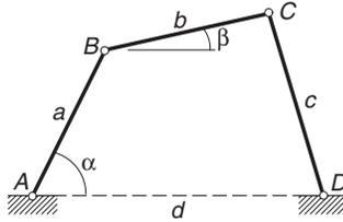
The linkage shown has the dimensions  $a = 100$  mm,  $b = 120$  mm,  $c = 150$  mm and  $d = 180$  mm. It can be shown by geometry that the relationship between the angles  $\alpha$  and  $\beta$  is
