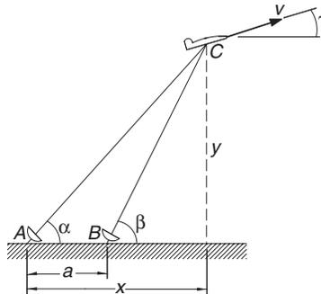
The radar stations  $A$  and  $B$ , separated by the distance  $a = 500$  m, track the plane  $C$  by recording the angles  $\alpha$  and  $\beta$  at one-second intervals. If three successive readings are
