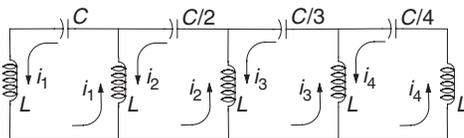
Determine the circular frequencies of oscillation for the circuit shown, given the Kirchoff equations
