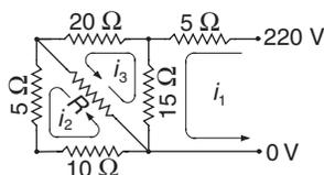
The electrical network shown can be viewed as consisting of three loops. Applying Kirchoff's law ( $\sum$  voltage drops =  $\sum$  voltage sources) to each loop yields the following equations for the loop currents  $i_1$ ,  $i_2$  and  $i_3$ :
