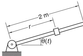
The system consisting of a sliding mass and a guide rod is at rest with the mass at  $r = 0.75 \text{ m}$ . At time  $t = 0$  a motor is turned on that imposes the motion  $\theta(t) = (\pi/12) \cos \pi t$  on the rod. The differential equation describing the resulting motion of the slider is
