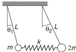
The two pendulums are connected by a spring which is undeformed when the pendulums are vertical. The equations of motion of the system can be shown to be
