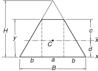
The trapezoid shown is the cross section of a beam. It is formed by removing the top from a triangle of base  $B = 48$  mm and height  $H = 60$  mm. The problem is to find the height  $y$  of the trapezoid that maximizes the section modulus
