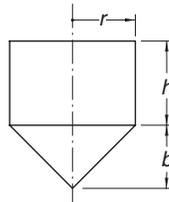
The cylindrical container has a conical bottom and an open top. If the volume  $V$  of the container is to be  $1.0 \text{ m}^3$ , find the dimensions  $r$ ,  $h$  and  $b$  that minimize the
